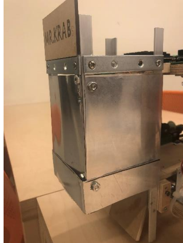
Figure 44. New Appearance of the Cone Holder After Cutting the Back Pillars
