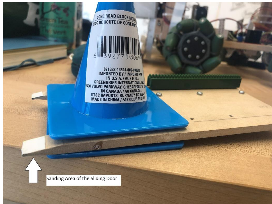
Figure 47. Illustration of How Sliding Door Hold Up the Upper Cone
